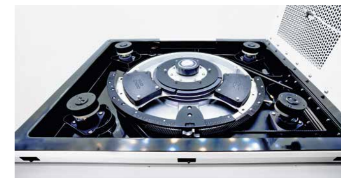
Eppendorf X-Drive with five eccentric mounting points and adjustable counterbalance provides dependable operation
